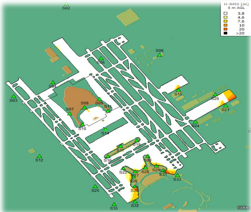
<Figure2.Multilateration(MLAT) Ground Station Installation Plan >
